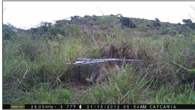
Fig 23: A feral cat enters a 'Havahart' cage trap with a disguised floor treadle trigger which ensures a humane catch method for feral or domestic cats.
