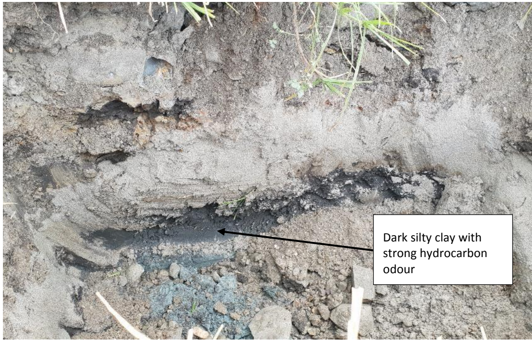
Photograph 3: TP06 showing odorous silty clay layer.
