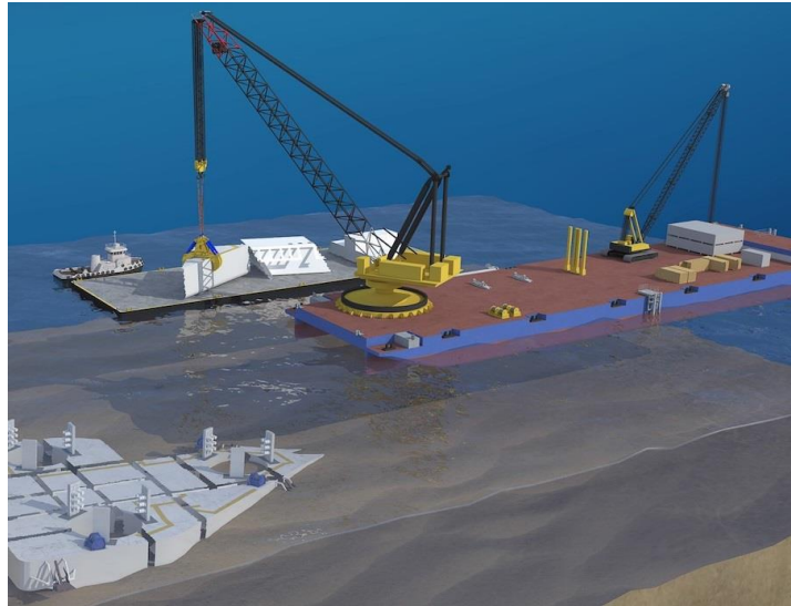
Figure 8 – Indicative cutting and removal operation, involving crane barge with rotating crane and support barge to receive scrap steel
