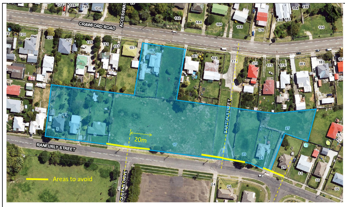
Figure 14 – Access Restrictions due to Intersection Separation Requirements
